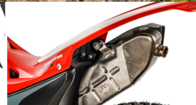
Enlarged exhaust, lightweight aluminum construction
