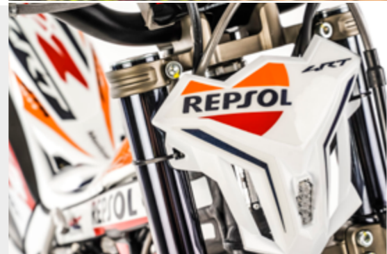
New triple clamps, machined from aluminum. Anodised in Titanium Grey
