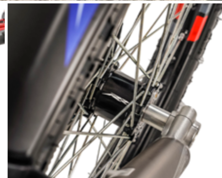
Lightweight hub, machined from aluminium
