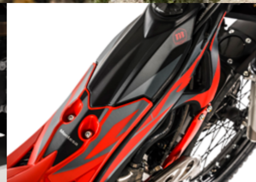
Aluminum fuel tank. New Montesa red-scheme decoration
