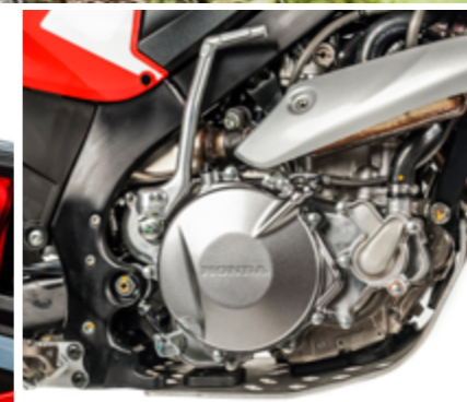
Fuel-injected four-stroke four-valve 259cc engine
