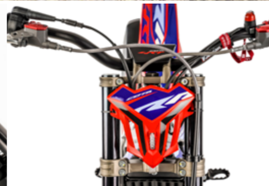
New triple clamps, machined from aluminium. Anodised in Titanium Grey
